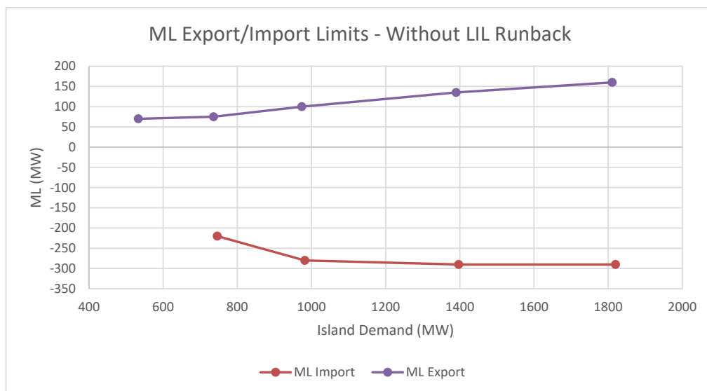
Figure 6–3. ML import/export limits, without LIL run-ups/runbacks or frequency control (no HRD units dispatched as generators)
